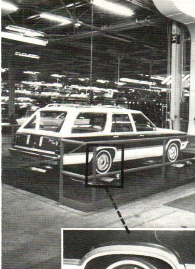
Testing for Unwanted Noises with the Burke-Porter Machine
