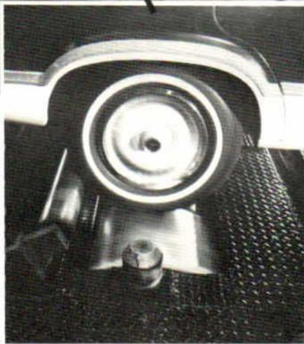
Testing for Unwanted Noises with the Burke-Porter Machine
