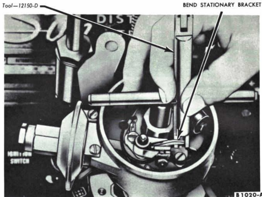
FIG. 7—Adjusting New Breaker Point Gap
