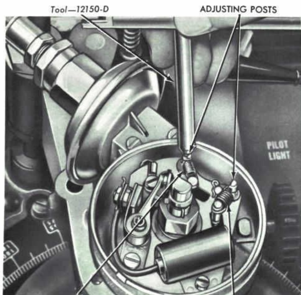
SECONDARY SPRING CONTROLS HIGH VACUUM ADVANCE
