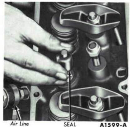
FIG. 27—Valve Stem Seal Removal or Installation
