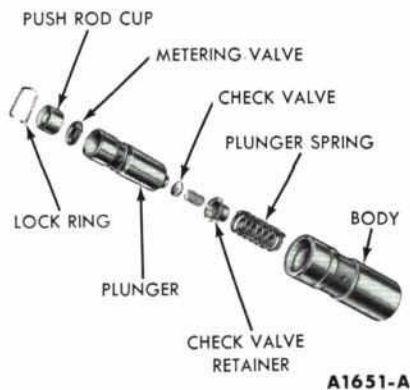
FIG. 40— Typical Hydraulic Valve Lifter Assembly
