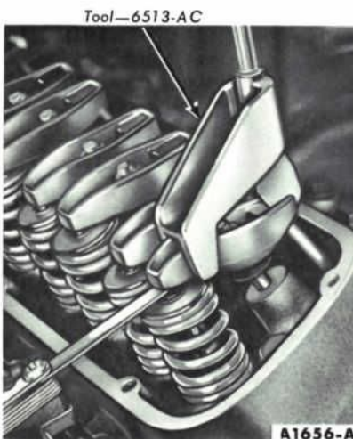
FIG. 17—Valve Clearance Check
