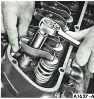
FIG. 16—Valve Clearance Adjustment
