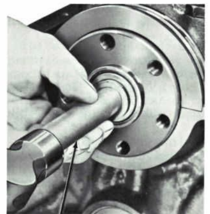
FIG. 49—Clutch Pilot Bearing Installation
