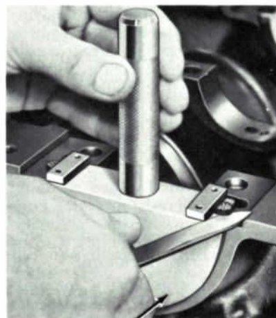
FIG. 54—Seal to Block Installation
