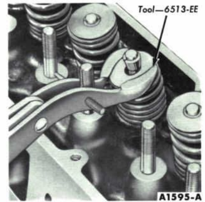
FIG. 23 — Compressing Valve Spring
