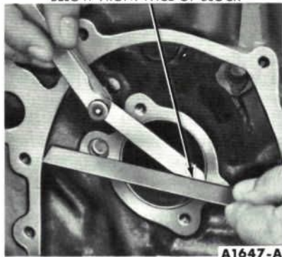
FIG. 58—Camshaft Front Bearing Measurement
