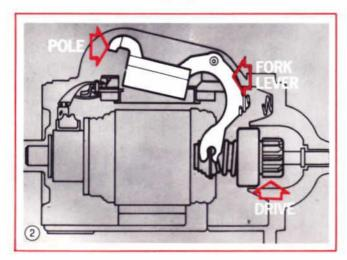
When the ignition key is turned to the START position, current flowing through the starter field coils sets up a magnetic action which acts as a pull-in coil to pull the metal pole piece into place. See Figure 3. When this occurs, the fork lever is pivoted and thus slides the drive pinion gear into contact with the ring gear. There is also a fine-wound hold-in coil (see Figure 4), to keep the pole in place during light loads or overrun.
