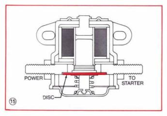
When these two terminals are bridged by the contact disc, current from the battery flows to the starter motor. On many starter relays there is also a fourth terminal labelled "I" for IGNITION. This terminal powers the ignition bypass circuit.
