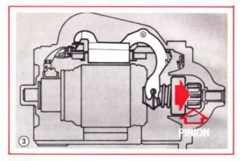
NOTE: If the hold-in coil were to open, the starter would still function but the movable metal pole piece would chatter during the overrun condition.
