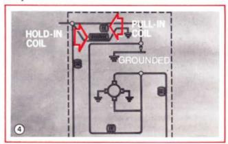
As the pole moves into place the drive pinion engages with the ring gear and the direct ground switch is opened. See Figure 5. Then all the field coils are energized normally to operate the starter motor. The motor begins to turn only after the drive pinion is engaged.
