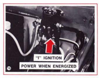
There is electrical power to this "I" terminal from the contact disc inside the relay but only when the relay coil is energized. There is no electrical power to the "I" terminal when the relay is de-energized (contacts open). See Figures 16 and 17.
