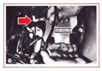
The other voltmeter lead connects to a good ground.
