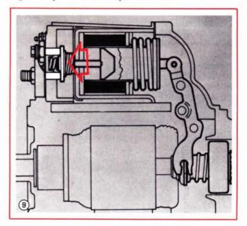
When a separate starter relay is used with this type of starter, there is a link installed on the solenoid to connect the battery terminal to the control terminal. See Figure 10. A replacement starter may or may not have this link . . . so be sure to transfer it if necessary.
