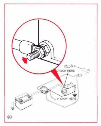
If no voltage is present but the relay "clicks" the relay should be replaced.
