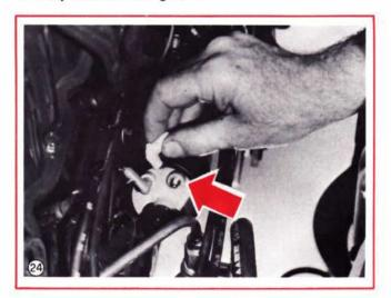
Crank the engine with the ignition OFF and carefully determine the exact reading on the voltmeter. Then, stop cranking the engine and insert the resistance of the carbon pile by turning the resistor control until the voltmeter indicates the EXACT SAME VOLTAGE as that obtained while the starter cranked the engine.
