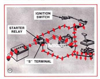
the starter. The starter connection to the chassis and the ground cable completes the load circuit to operate the starter.
