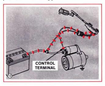
The moment the drive pinion engages with the ring gear, the main contacts in the solenoid are closed. Battery current then flows through the starter motor and the engine begins cranking. See Figure 13.
