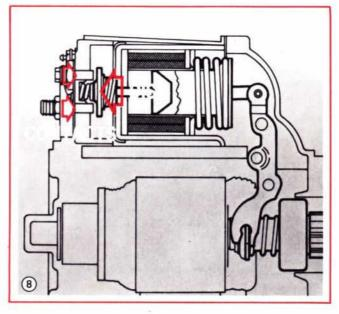
Thus the solenoid in this type of starter functions as a starter relay as well as a drive actuator. The unit does not require a separate starter relay.
