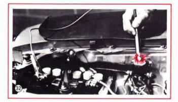
NOTE: Remember that in combination floor-shift automatic transmission equipped passenger cars, there is a neutral switch in the starter circuit that may be out of adjustment or worn. If you have power to the neutral switch but no power away from it, you'll have to adjust the switch. When the switch is set properly, you will get a positive continuity test through it ... both in PARK and NEUTRAL positions of the shift lever.
