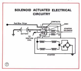
The solenoid also has a set of load circuit contacts and a contact disc similar to the ones used in a starter relay. See Figure 8. In addition, it may have an extra terminal for the ignition bypass circuit.
