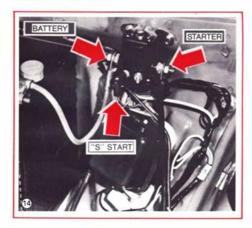
When the relay coil is energized from the START terminal (electrical circuit completed by the ignition switch in the START position) the solenoid core pulls a heavy contact disc across the large terminals. See Figure 15.
