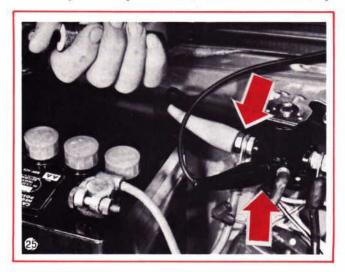
However, if the draw is HIGH . . . it indicates a short circuit in the starter motor or a mechanical binding condition. Check the cables for a grounded condition and if they appear normal, the starter should be removed for a complete visual inspection and bench testing.
