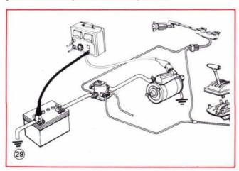
NOTE: Any voltage drop that is HIGHER than specifications indicates there is excessive resistance.
