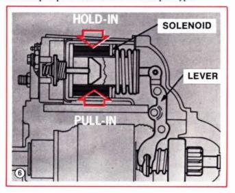
This solenoid coil contains two windings . . . a pull-in winding and a hold-in winding.
