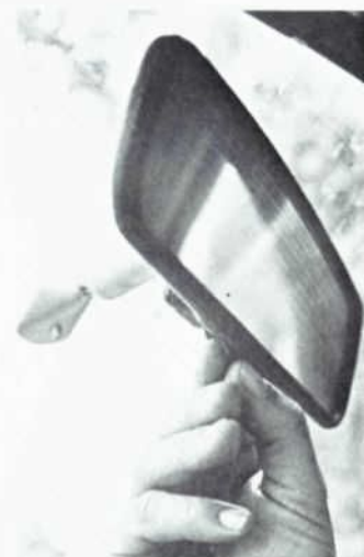
After 5 minutes, secure mirror to mounting bracket. Ultimate strength develops in 24 hours.
