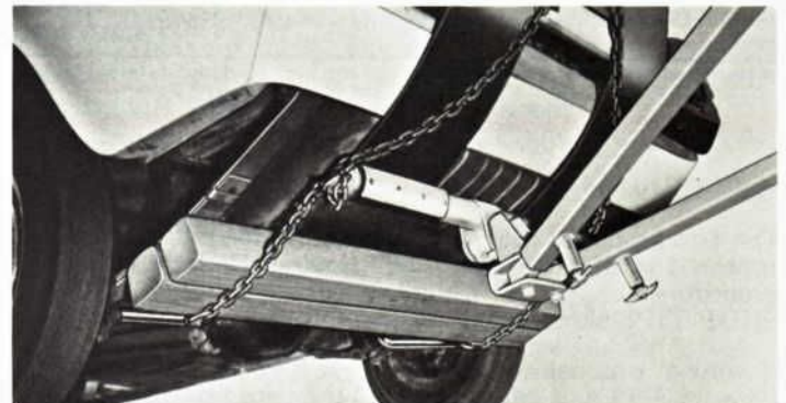
To tow the Mustang by the rear end, the chains are hooked around the rear axle housing. Before lifting, 4 x 4 wood beams approximately 55" long should be placed between the chains and the underside of the car.
