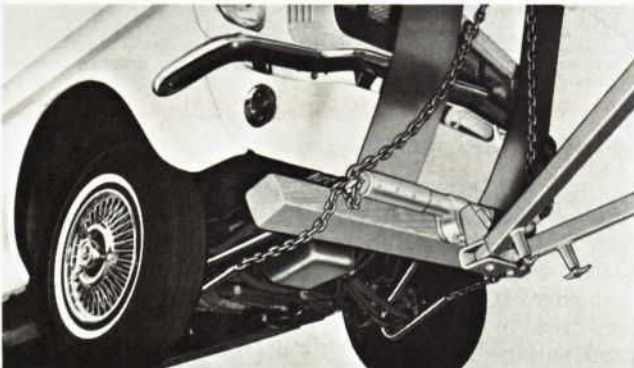
Front spacers in the above photo are 4 x 4 wood beams approximately 55" long. It is important that they rest on the body rails just behind the body lower panel.
