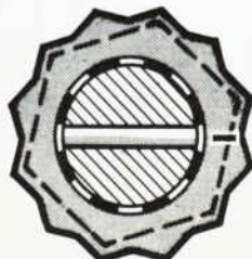
INSTALL LOCK ON NUT SO THAT CASTELLATIONS ARE ALIGNED WITH COTTER PIN HOLE.
