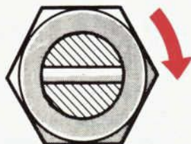
WITH ROTOR AND WHEEL ROTATING, TORQUE THE ADJUSTING NUT TO 17 - 25 ft. lbs.
