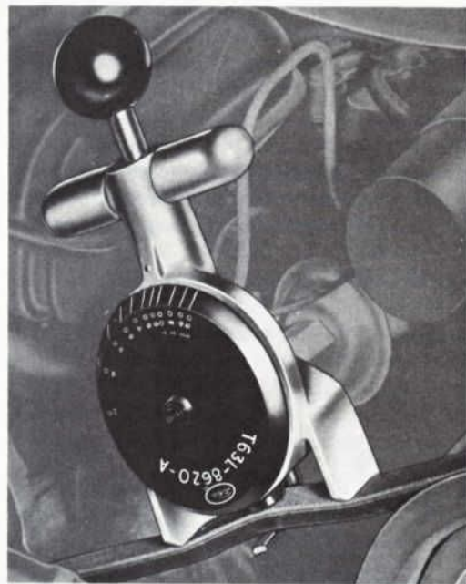
Checking For Proper Belt Tension
