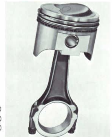
Figure 3—Impact-extruded Piston and Special Connecting Rod
