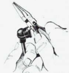
Figure 4—Crimping Hairpin Terminal
