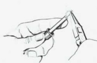
Figure 3—Installing Hairpin Terminal
