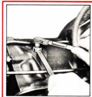
Figure 12—Adjusting FMX Rear Band Externally, (Late Ford-Fairlane-Montego Models) When There is No Access Hole In Floor Pan
