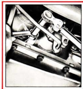
Figure 14—Adjusting the C4 Intermediate Band Externally With a Special Tool
