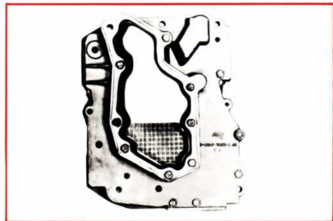
Figure 8—The C4 Filter Screen Attached to Lower Valve Body by Machine Screws
