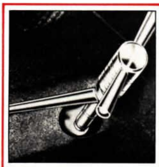
Figure 11—Adjusting FMX Rear Band Externally Through Access Hole in Floor Pan—Typical. (Early Models.)
