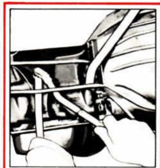
Figure 13—Adjusting FMX Rear Band Externally, (Late Model Mustang and Cougar) When There is No Access Hole in Floor Pan
