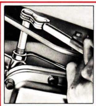
Figure 15—Adjusting the C4 Low-Reverse Band Externally With a Special Tool
